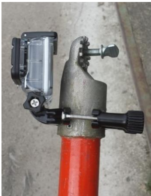
Installation of camera on insulation rod.
